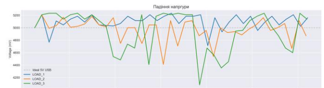
Fig. 2. Voltage change graph under physical load for SG90
